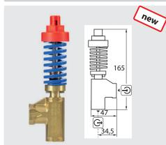
$\bigcirc$  = Inlet 1/4" F.  $\bigcirc$  = Outlet 3/8" F. Min. 200 bar, max. 700 bar / 60 °C, short-term max. 85° C
